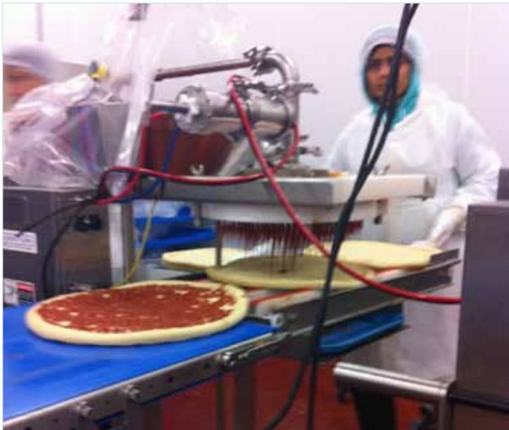
Pace Processing - Automated application of sauce on pizza dough
